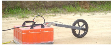
Ground-penetrating radar unit used to image subsurface
