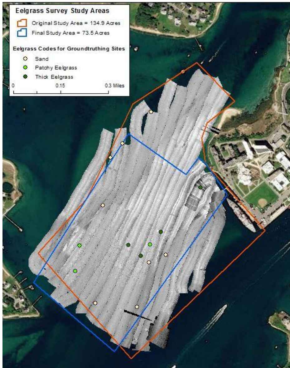
Figure 10. Side scan sonar mosaic and groundtruth points from pilot study in 2018 at the MMA impact site.
