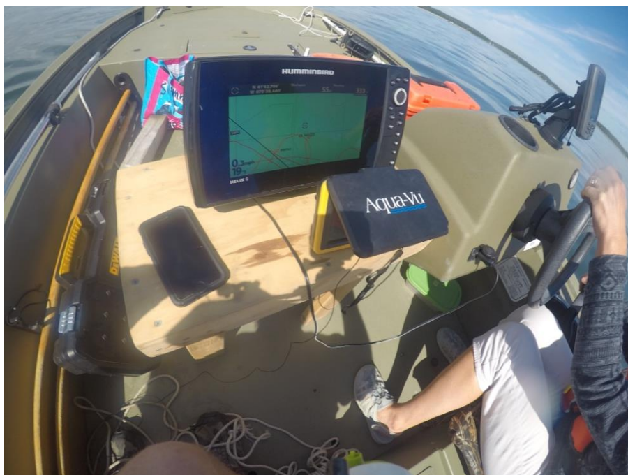
Figure 3. Humminbird Helix9 side scan sonar onboard the R/V Flatfish
